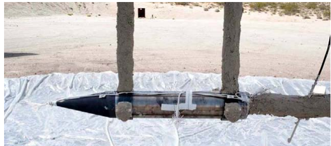
FIGURE 2. Liquid Fuel Fire Test Setup of CHFD Test Article.
