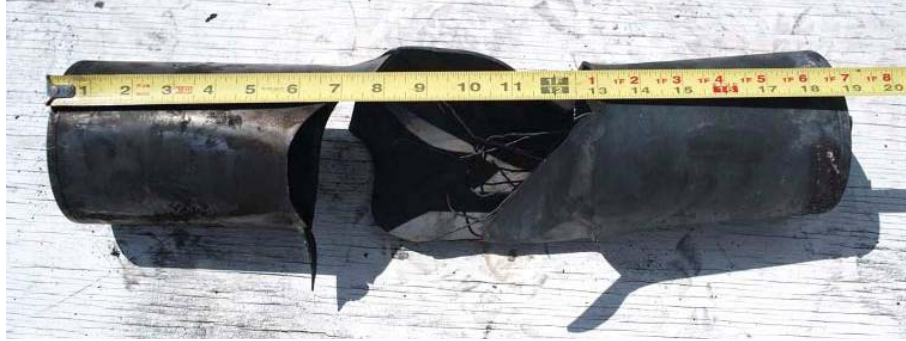
Figure 18. Fragments Collected from Liquid-Fuel Fire Test.
