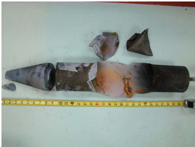
FIGURE 19. Three Recovered Fragments from 3.81-cm Bore Diameter With Fielded Propellant.
