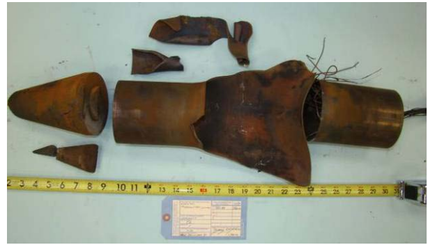
FIGURE 12. Four Metal Fragments Recovered from Test Asset 3.
