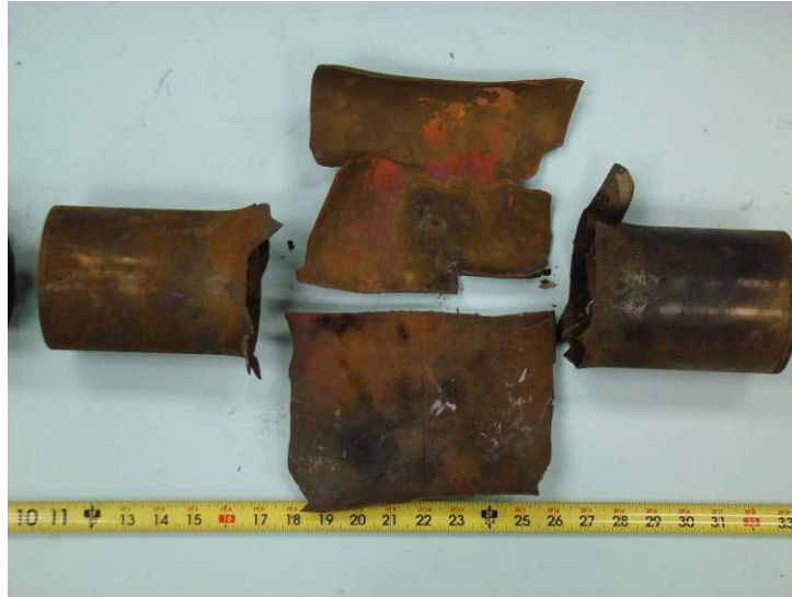
FIGURE 15. Four Recovered Metal Fragments from 1.27-cm Bore Diameter.
